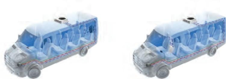
Evaporator vertical on the side at the rear
