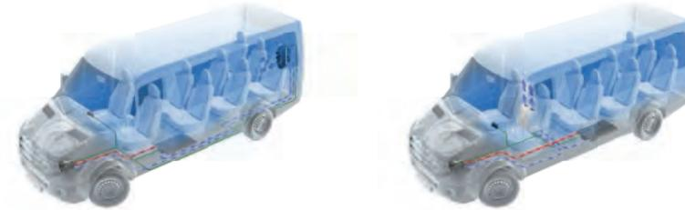
Evaporator vertical on the side at the rear
