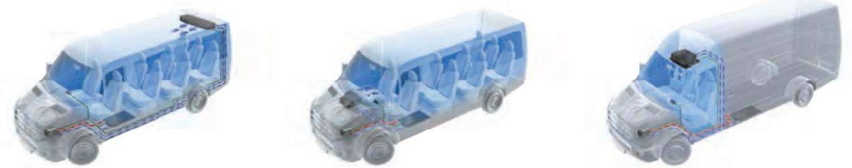
Evaporator under the roof
