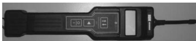
Fig. 7-8 Electronic leak detector
